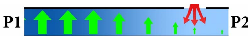
Fig. 6 – The model of the sidestream sampling line, with the breach in wall. When the P_{ins} < P_{atm} during expiration, the suctioning of the atmospheric air occurs.
